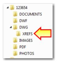
The use of temporary XREFs is allowed. However, when the temporary XREF is no longer needed, DETACH the temporary XREF properly through the External Reference Manager.
