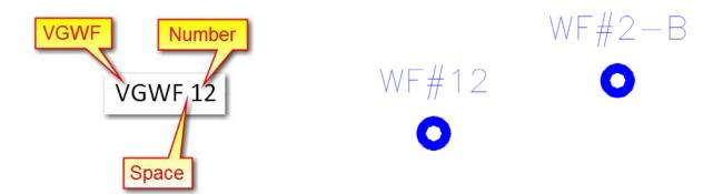
When using the wetland flag code, the Wetland Flag symbol and text label will be placed onto the EX-SV-WETL-TEXT layer separate from the Wetland Line layer, EX-SV-WETL.
