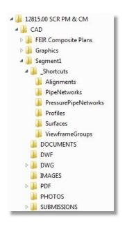
All survey base drawings (DWG files) containing either Civil 3D alignments or Civil 3D surfaces that are intended to be referenced through Data Shortcuts shall be first copied to the Segment#/DWG/SV
