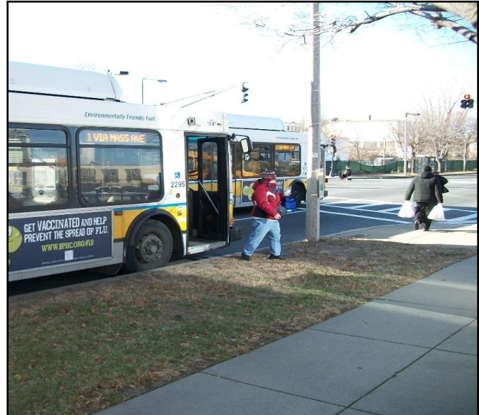
Bus stop Without Accessible Landing Pad or POT
