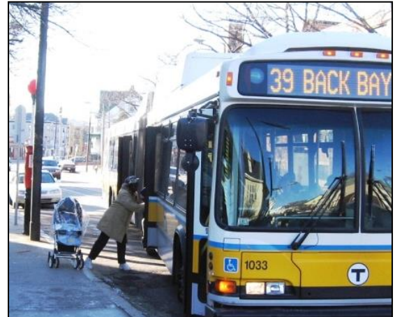
Bus Back Door Not Aligned With Curb
