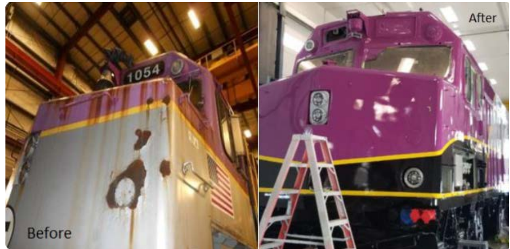
Before/after photos of F40 locomotive overhaul
